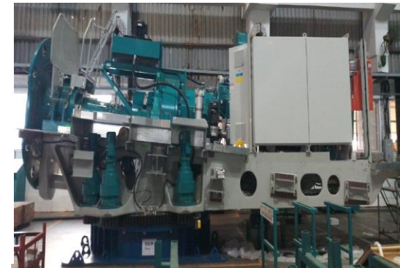
S120 Nacelle Assembly at Plant
