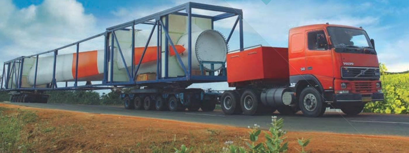
the blade has been challenging due to constrained road conditions. The logistics team at Suzlon developed an innovative two fold transport system, which used a specialised 'Adapter Trailer' for the first time in India. This innovative approach ensured unbound manoeuvrability through the hilly terrain, while transporting long blades safely in a cost-effective and time-efficient manner to the most remote wind sites.
