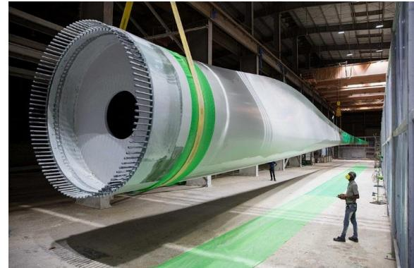
Suzlon SB 63 blade being inspected at Padubidri factory
